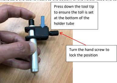
4. Place the high adjustment jig under the creasing tool position and insert the creasing tool holder (Make sure the cylinder is in Down position).
