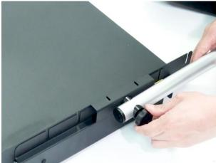
8. Hang the media collection tray onto the connecting holder and tighten it up with hand screw.
