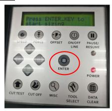
**Step 9** Go to "MISC" menu, use arrow left/right keys to select "Adjust Paper" and press "ENTER" key. Set the "Adjust Paper" to 22.5mm and press "ENTER" key to confirm.
