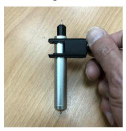
Make sure the tool is insert to the bottom of the holder tube and turn the hand screw to lock its position
