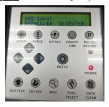
Step 11 Then use arrow up/down keys to define the repeated value (value =  $0^{-500}$ ) and press "ENTER" key.
