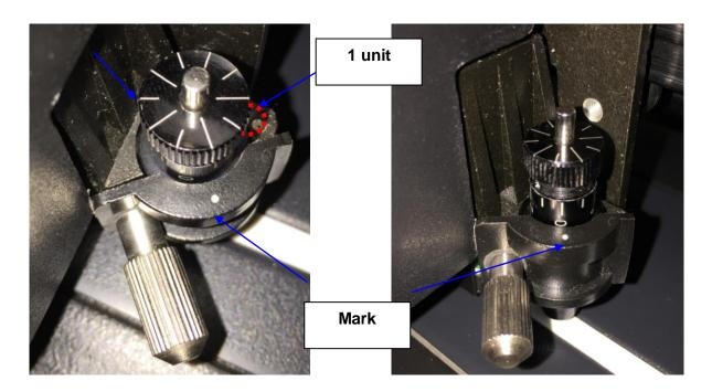
There are 10 units on the scale; each unit equals to 0.05 mm, allowing you to adjust the blade length for 0.00mm-5.00mm.
