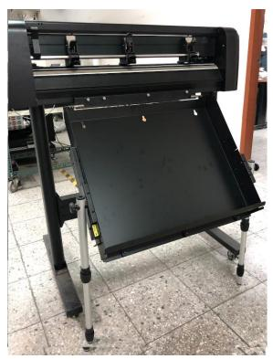
Note: Drawer-type autofeeder design allows users to extend the feeder to accommodate B2 size paper.
