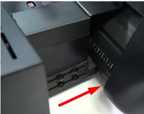
5. Loose the screw on the rear platen.
