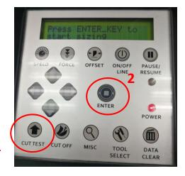
The default cutting force and offset value of the cutting test are 80gf and 0.275mm respectively. Press [ARROW KEY] to move the tool carriage to the position where you like. Then, press the [ENTER KEY] to perform Cut Test.
