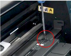
2. Tighten the thumb screw to fix the connecting brackets to the side plate of the Jaguar V/RXII.
