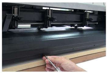
6. Fix the connecting bracket on the rear platen with screws.
