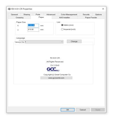
**Paper Size (Paper Page) [DEFAULT SETTING:** Y = the width of machine; X will be automatically set to be twice the length of Y]
