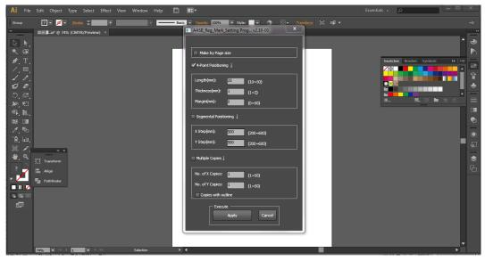
Step 5 Four types of registration marks are introduced here: 2-Point Positioning, 4-Point Positioning, Segmental Positioning and Multiple Copies.
