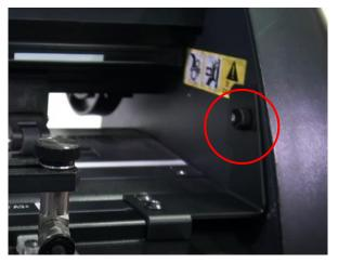
3. Loose the screws on the side brackets of auto feeder.
