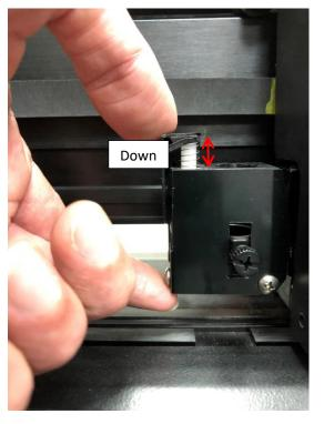
Press the cylinder by hand and hold the bottom to ensure the VCM to be hold while pressing. As shown on above pictures.
