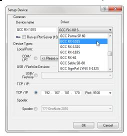
Step 4 Input the IP address you had acquired from the control panel to the TCP/IP. Click OK to complete settings.
