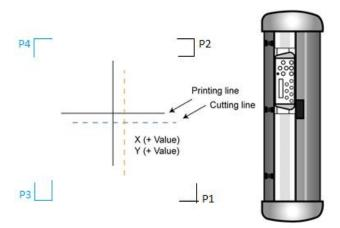
The setting in Paper Feeder Page works when 2-point positioning registration mark setting is applied in a cutting file. Please refer to A-4 Add Two Point Registration Marks section or A-5 Add Two Point Registration Marks section.
