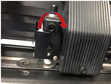
Completed. Dis-engage the crease tool holder and reboot the machine and size to check.
