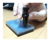
**Step 3** Adjust the blade tip to suitable length by screwing "Blade tip adjustment screw" clockwise or count-clockwise.
