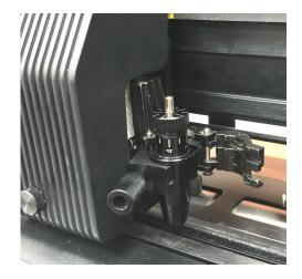
Step 2 Fasten the thumb screw to fix the tool carriage.
