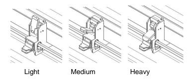
Please note that the pressure of the pinch rollers on the left and right sides should always be the same or heavier than the pinch rollers in the middle. The pressure of the pinch rollers on the left and right sides should be set to the same pressure setting. You can use the following combinations of the pinch rollers.
