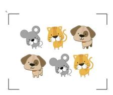
\*Registration Marks: set the distance between the edge of the material and the registration marks in Mark Offset; set the size of marks in Mark Size; set the line thickness of marks in Mark Thickness.
