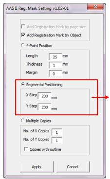
For precise cutting quality, it is suggested to select "Segmental Positioning" when you are working on an extra long or large-sized image to increase cutting accuracy.
